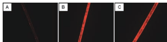
Figure 4. Fluorescence microscopic images of a polymerized and heat-treated sulfonated PS fiber, obtained after 2 (A), 4 (B), and 6 (C) deposition cycles.
